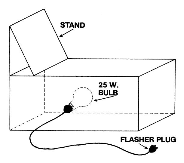
In order to make one of these miraculous instruments you will need a box, an old shoe box will do; a twenty five watt light bulb; a light socket with wire and plug attached (available at any hardware store) and a flasher plug (also available in any hardware store with the exception of those in Queensland, Australia and don't ask me why) and a sheet of wax paper.
